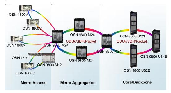
Figure 1-2 Position of the OSN Series on the entire network
